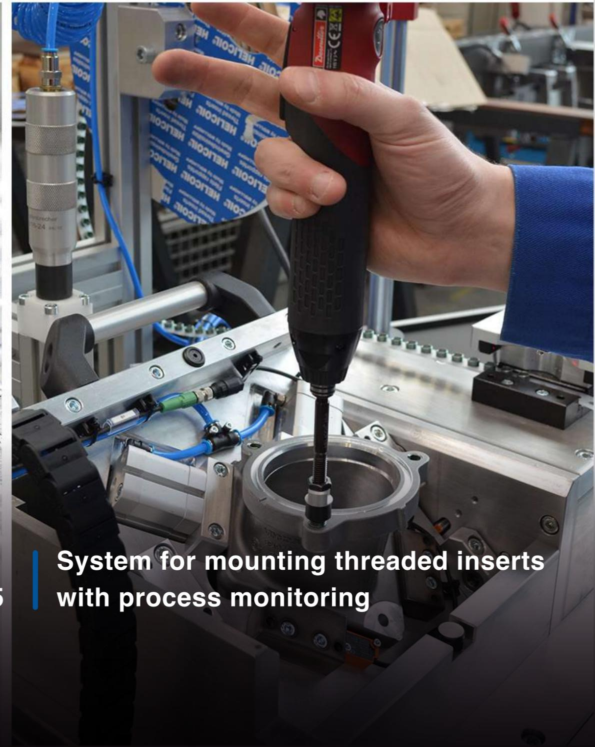
**System for mounting threaded inserts with process monitoring**
