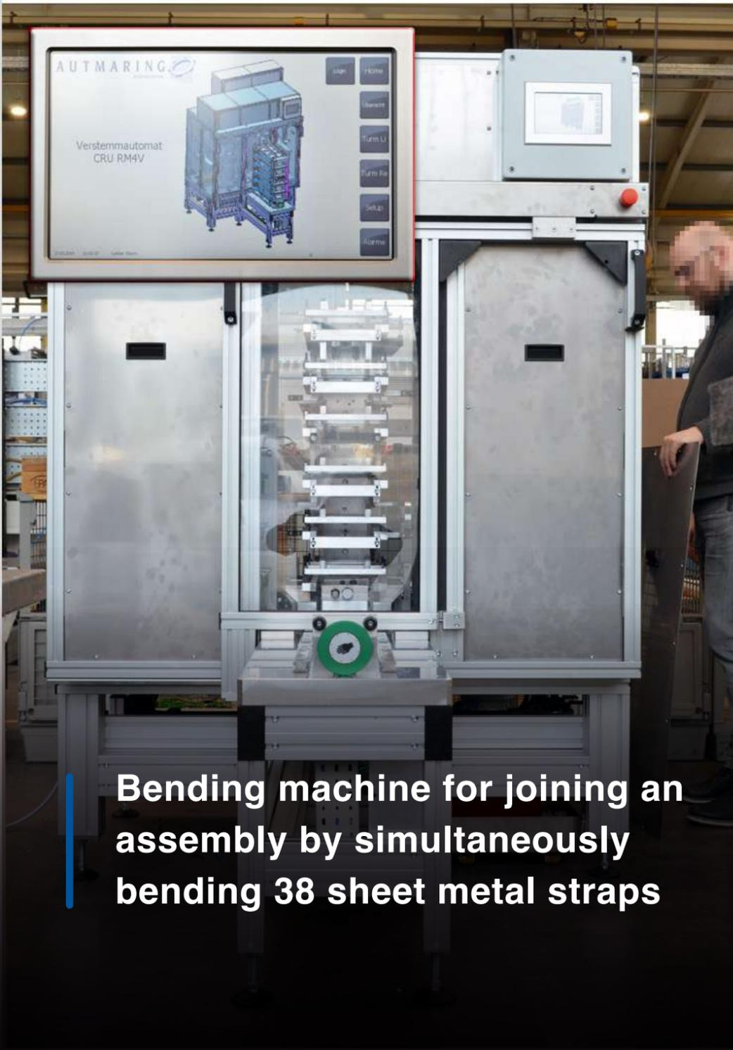
**Bending machine for joining an assembly by simultaneously bending 38 sheet metal straps**
